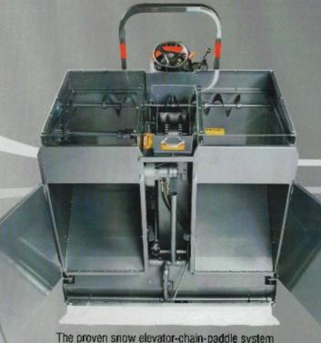
The proven snow elevator-chain-paddle system moves the scrapings from the ice to the snow bin effortlessly. The wide rear-access doors on the OLYMPIA\*\* 250's snow bin allows for ease of dumping.
